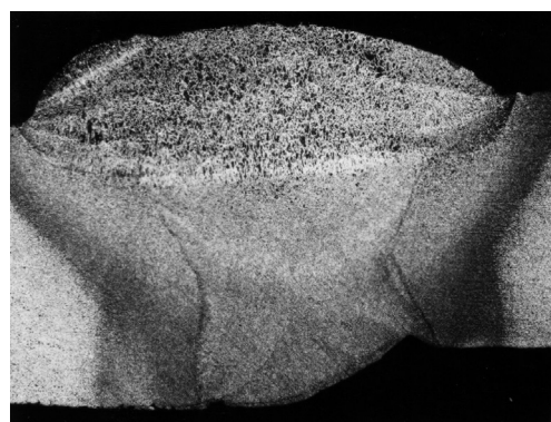
Fig. 4. Pipe weld joint, outside of damage
